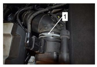
Remove low pressure hose <1> from air filter • housing.
