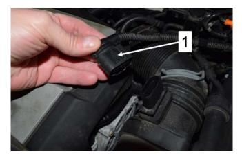
Reinstall air duct hose in the direction of the • <arrow> and reinstall the clamp.
