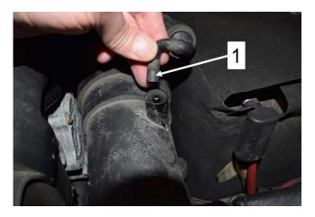
Reinstall low pressure hose <1> onto air filter housing.
