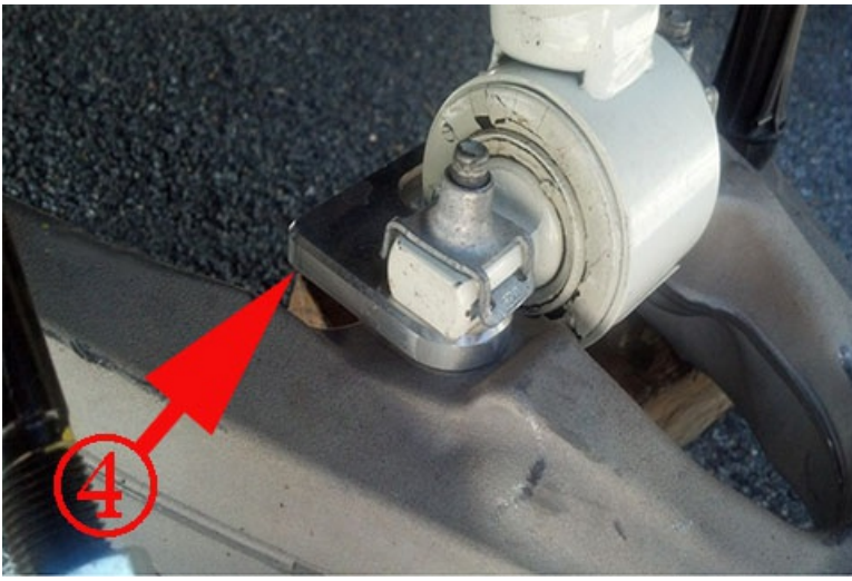
4. Aftermarket lift kit blocks installed
