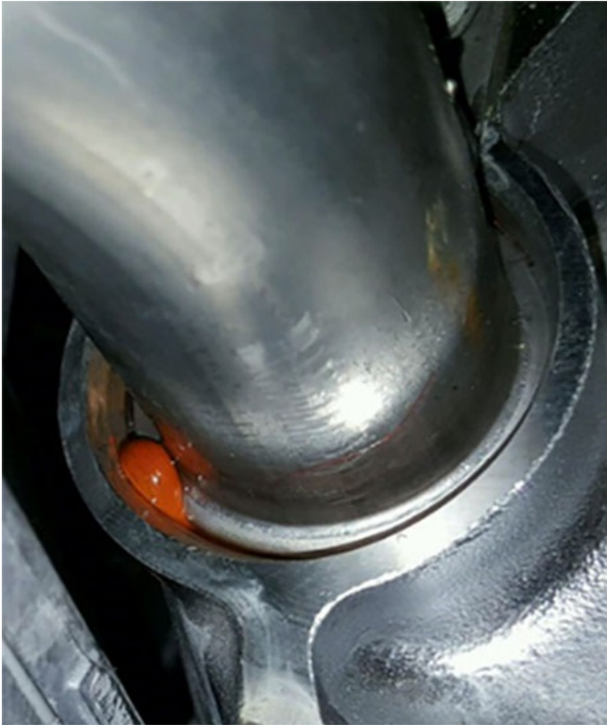
View of a rolled or pinched O-ring at Exhaust Gas Recirculation (EGR) coolant feed pipe. Refer to call out #2 in the above picture.
