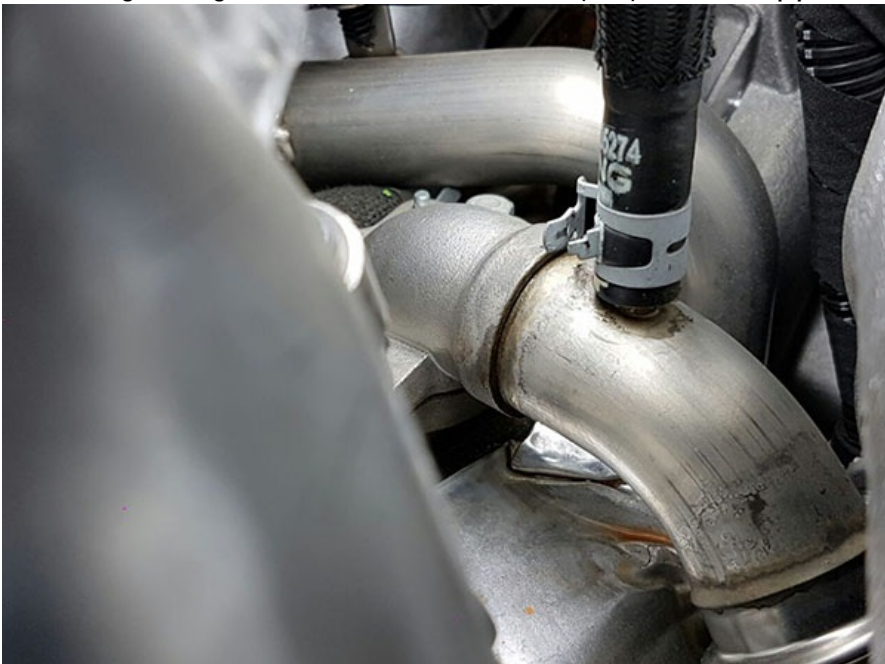
Another view of the leaking welded flange on the Exhaust Gas Recirculation (EGR) coolant feed pipe. Refer to call out #2 in the above picture.
