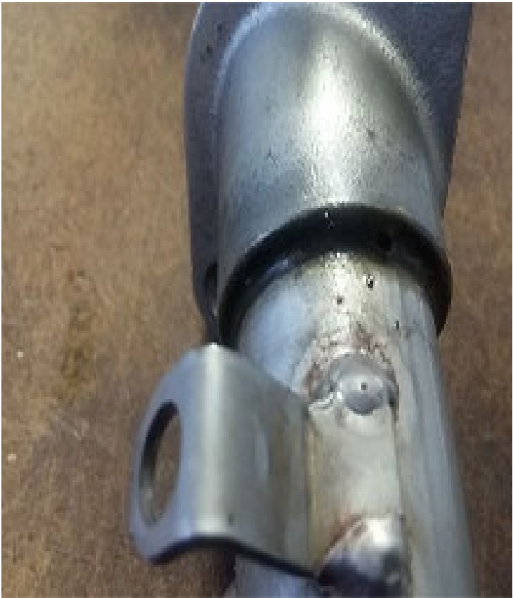
Welded flange leaking on the Exhaust Gas Recirculation (EGR) coolant return pipe. Refer to call out #1 in the above picture.
