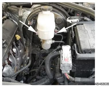
2. Locate the brake master cylinder nuts.
