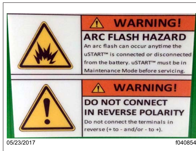
Fig. 4, Ultracapacitor Warning Labels
