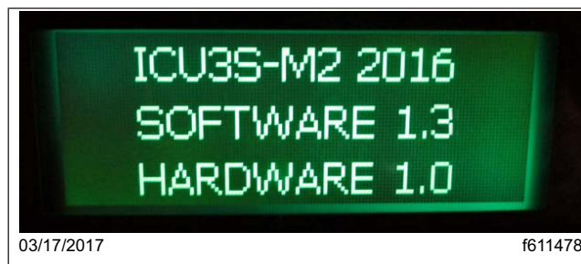
Fig. 1, ICU3S Screen Showing Software Version 1.3 (correct)
