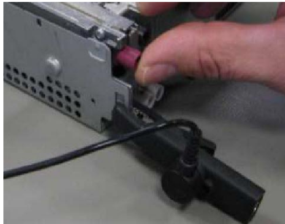
Figure 7. Alligator clip on MMI housing.
