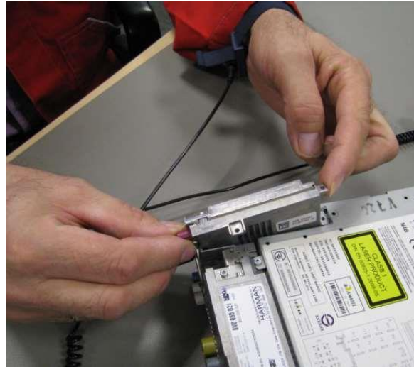
Figure 11. Remove the top out first.
