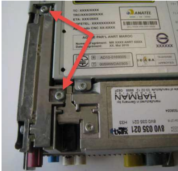
Figure 13. Do not over torque screws.
