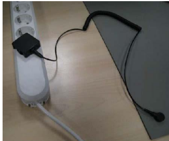
Figure 4. Grounded ESD Work Surface.
