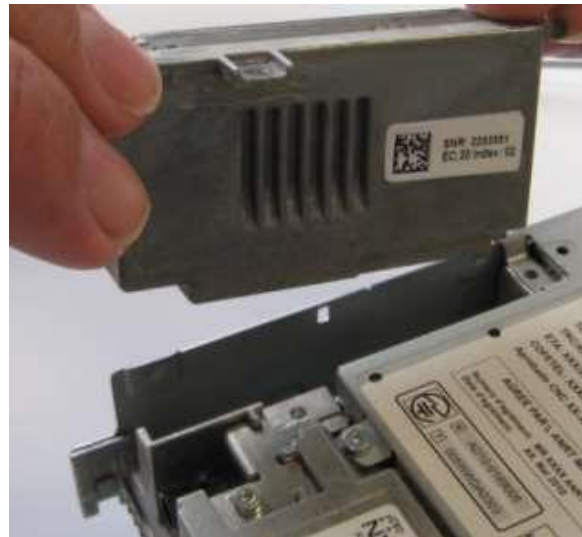
Figure 12. Insert the new telephone module.
