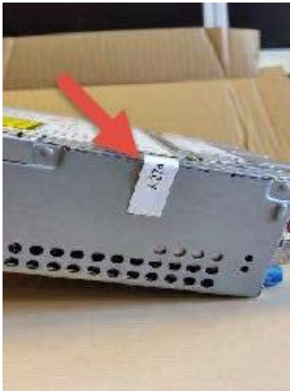
Figure 14. Apply new warranty label.
