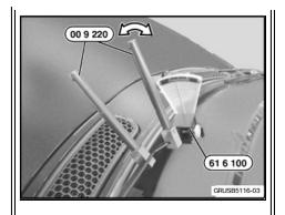
2. If out of adjustment, use tools shown to align wiper arm.
