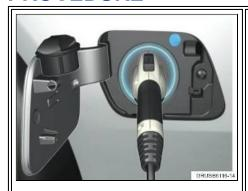
1. Connect Level 2 (220V) charging cable to the vehicle.
