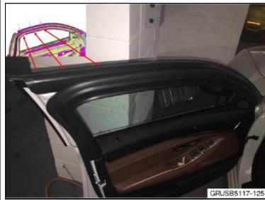
3. Apply adhesive tape on the window frame (83 19 0411397 – Fabric tape, Tesa 4657) at the 3 positions shown.
