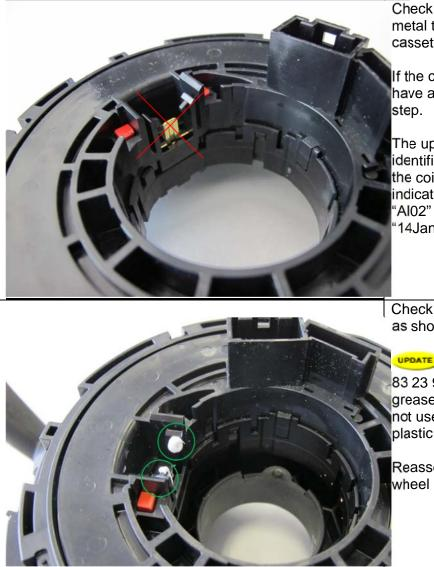
Check the coil spring cassette for a metal tab as shown. If the coil spring cassette has a tab, replace it.
