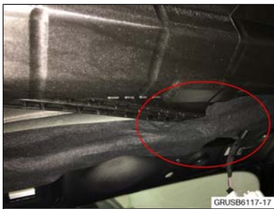
G. Check to the right of the passenger front vanity light above headliner.
