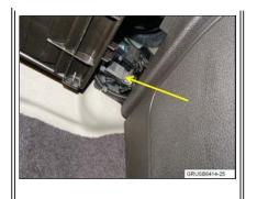
7. Locate the MOST bus access point in the passenger's side footwell near the bulkhead. Remove the connector piece from the securing bracket.
