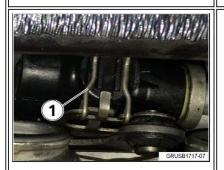
Disconnect the clamp holding the transmission oil cooler thermostat from the holder (1)
