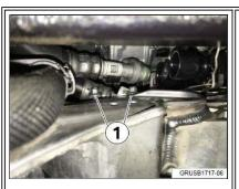
Remove the two 8mm bolts (1) that hold the thermostat bracket to the sub-frame. Replace the bolts (PN 34 30 6 771 214) during installation and tighten to 8 Nm.
