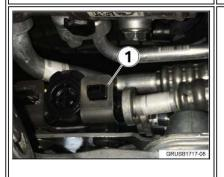
Slide the holder out from the transmission oil cooler thermostat (1).
