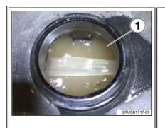
Inspect the cooler lines for contact with the left front output shaft (1). Replace the cooler lines if the CV boot has cut into the lines. Replace the inner CV boot if it is damaged (Reference Repair Instruction 31 60 535 "Replacing two gaiters on output shaft").
