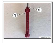
The illustration describes the proper engine oil level when using the engine oil dip stick.
