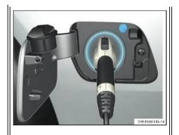
2. Connect Level 2 (220V) charging cable to the vehicle.
