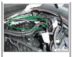
Proper location of the fuel line (behind the tank ventilation hose).
