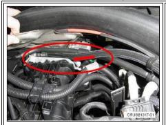
Picture shows incorrectly positioned fuel line (in front of the tank ventilation line) contacting the rear bracket of the intake manifold.
