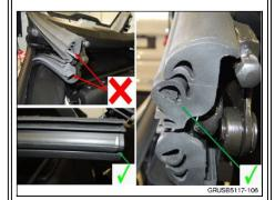
4. Push inserts the rest of the way into the seal as shown  $(\sqrt{})$
