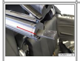
2. Place inserts part-way into end of convertible top seal (both front and rear seal), adhesive end last.
