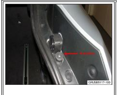
1. Adjust the bump stop height. Refer to repair instructions REP 51 23 ...Adjusting/replacing bump stops (accessible in ISTA via Group/Subgroup 4162).
