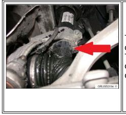
The front suspension ride height has been reduced on one or on both sides. The front spring strut damper slips through the clamp of the steering knuckle, damaging other front end components.
