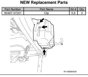
c) Reinstall the height control compressor cover with the 3 **NEW** clips.
