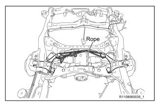
c) Fix the upper arm with a rope etc. to restrain expansion of the upper arm in order to prevent the drive shaft from coming off.
