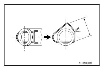
2) Spread the clip and slowly pull the height control tube straight out.
