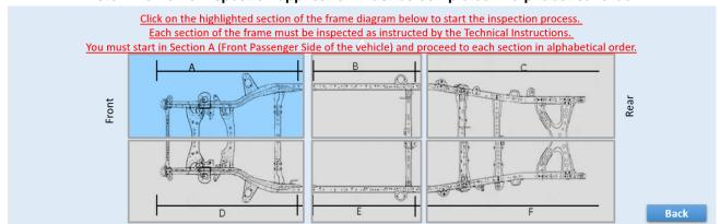
c. Inspect the frame section and inspect all surfaces of the frame rail and crossmember. Select the photo that best represents the frame condition. If perforation of 10mm or larger is identified select "Peroration of the Frame".
