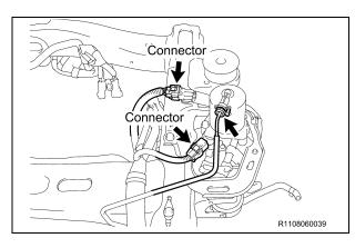
b) Disconnect the 2 connectors and tube.
