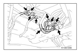
b) Disconnect each connector and clamp.
