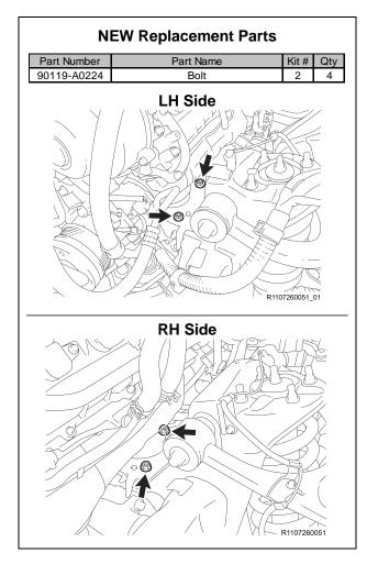
b) Attach the engine mounts with the 4 **NEW** bolts and torque to spec.
