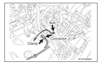
c) Disconnect the skid control sensor connector and clamp.
