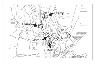
b) Reconnect the ground wire with the bolt and torque to spec.
