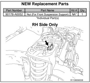
d) Reinstall the bracket with the **NEW** nut and torque to spec. **(W/AIR SUSPENSION, RH Side Only)**
