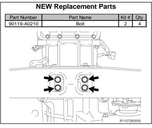
c) Attach the transmission mount with 4 **NEW** bolts and torque to spec.
