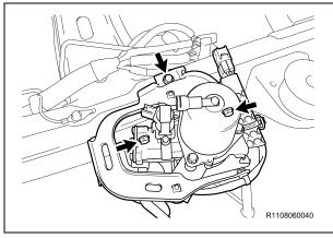
c) Remove the 3 bolts and No.1 height control compressor assy.
