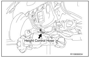
7. RECONNECT THE HEIGHT CONTROL HOSE (W/ AIR SUSPENSION)
