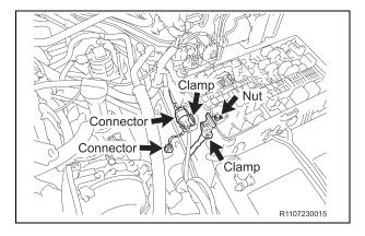
c) Reconnect the (+) positive battery cable with the nut and torque to spec.
