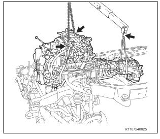
c) Remove the engine and transmission assy.
