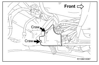
b) Reinstall the connector cover and reconnect the 2 craws.
