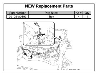
b) Reinstall the breather tubes with the **NEW** bolt and torque to spec.
