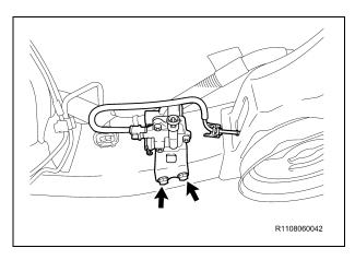
c) Remove the 2 bolts and No.2 height control valve subassy.
