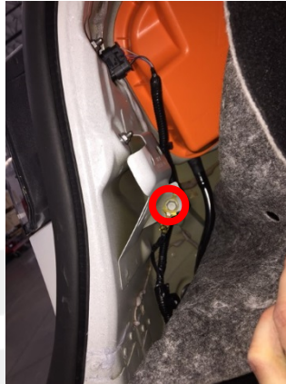
Figure 5 (LH rear quarter terminal)
