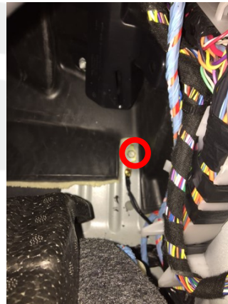
Figure 10 (RH toeboard terminal)
