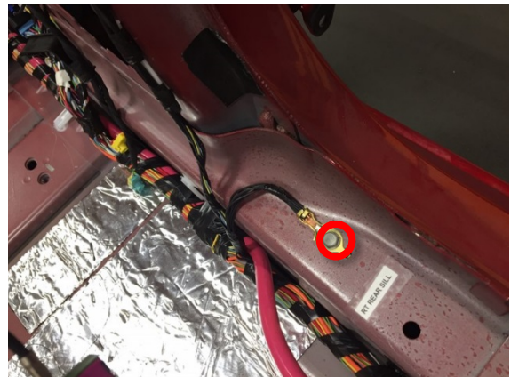
Figure 8 (RH sill terminal)
