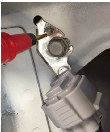
Figure 11 (measure on ground terminal metal)
