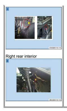
3. Using appropriate tool, slightly dent the body panel at the indicated spot (X) to eliminate flexing.
