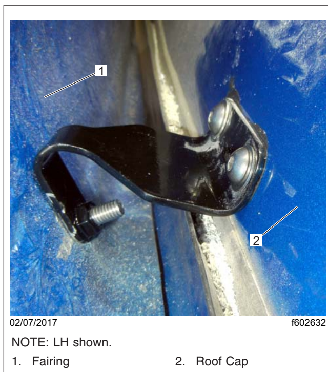
Fig. 13, Fairing Bracket Installed
