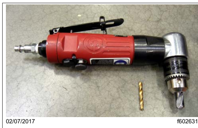
Fig. 10, Right-Angle Drill and Cut-Off Drill Bits
