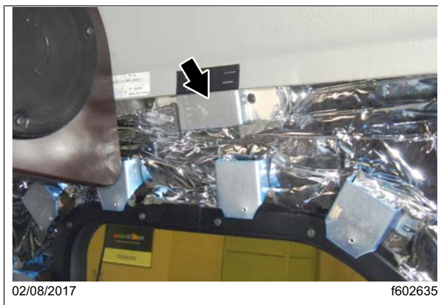
Fig. 15, Headliner Standoff Bracket Installed in New Location
