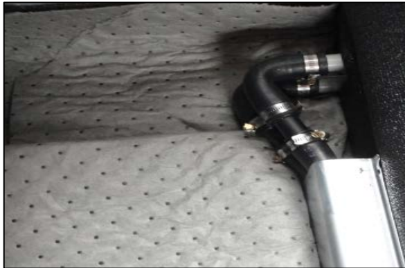
Figure 4, Place absorbent pad under the hoses
