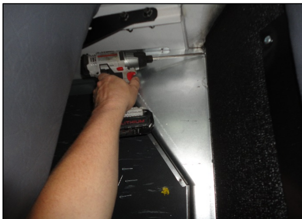
Figure 3, Removal of interior heater hose cover
