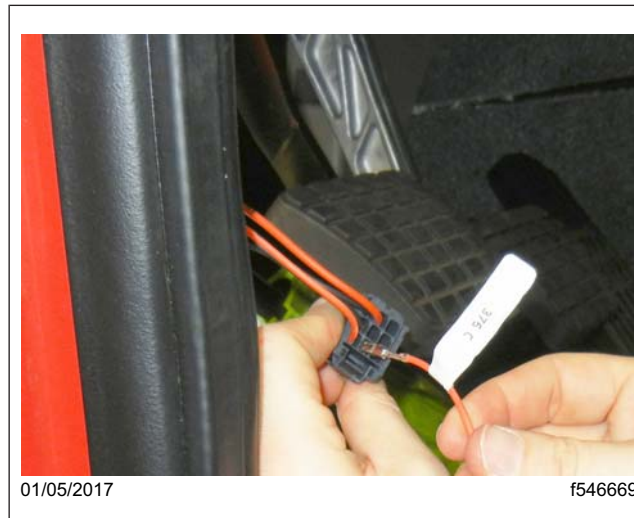
Fig. 10, Circuit 376C into Connector 52B
