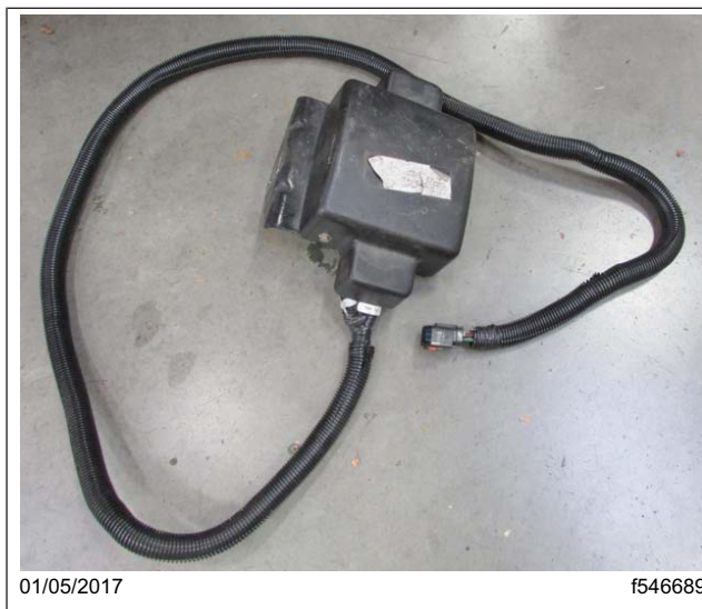
Fig. 30, CPDM Removed from the Vehicle
