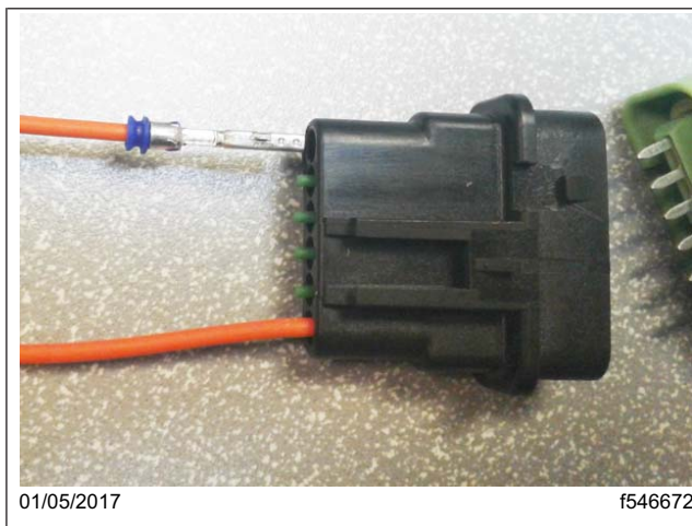
Fig. 13, Splice Pack Terminal Insertion
