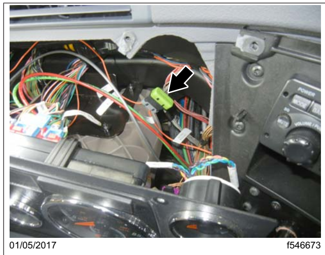
Fig. 14, Splice Pack Routing
