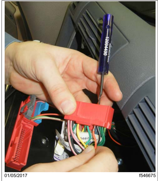
Fig. 16, Wire Removal from Cavity D12 of ICU Connector 2A
