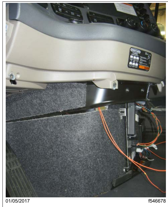
Fig. 19, Routing the Wires to the ABS Module (FL721-A installation shown)
