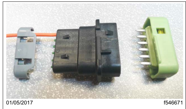
Fig. 12, Splice Pack Cover and Lock (removed)
