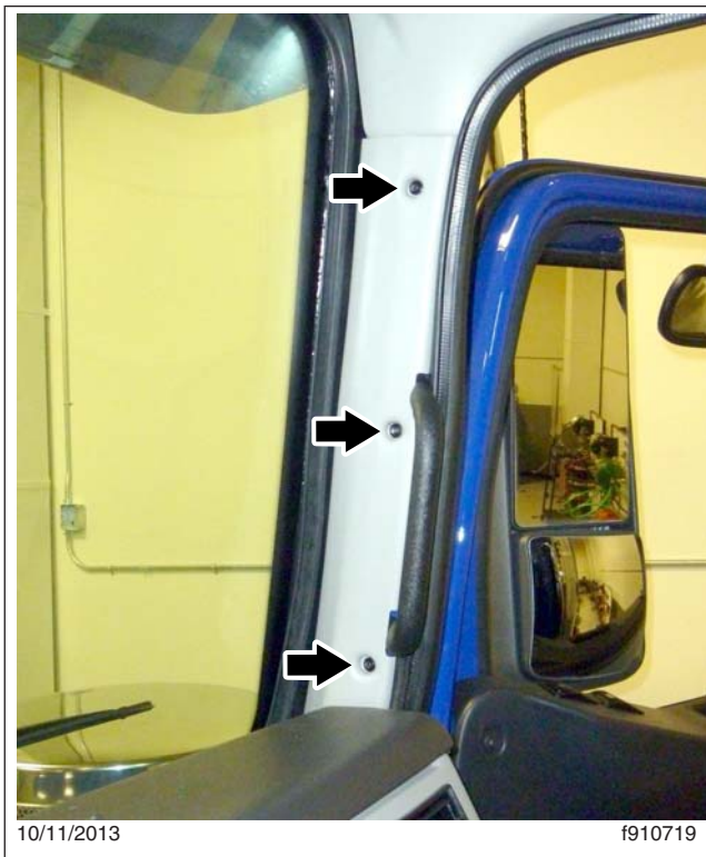
Fig. 3, A-Pillar Cover Screws
