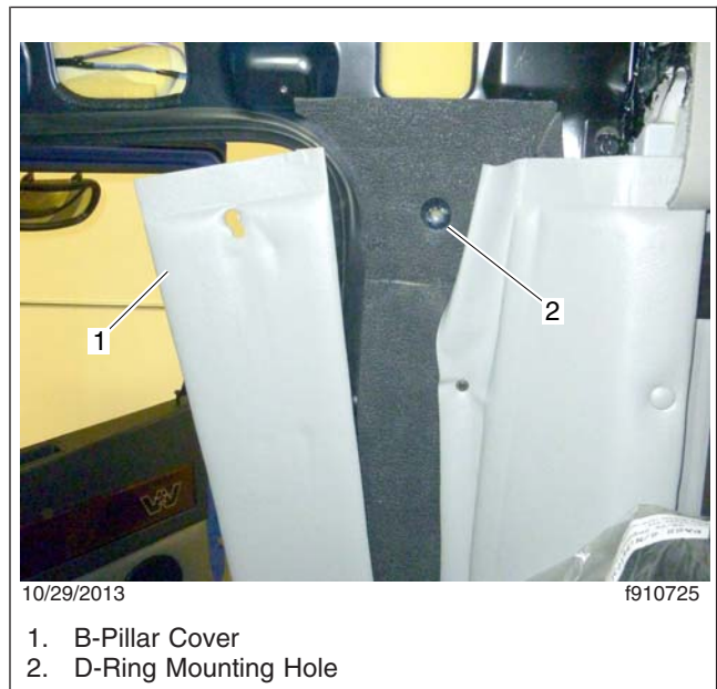
Fig. 7, B-Pillar Cover, Unfastened
