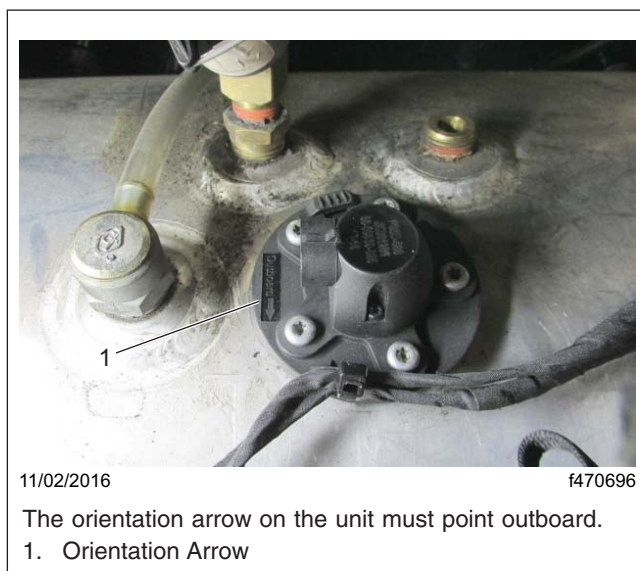
Fig. 4, Sending Unit Orientation
