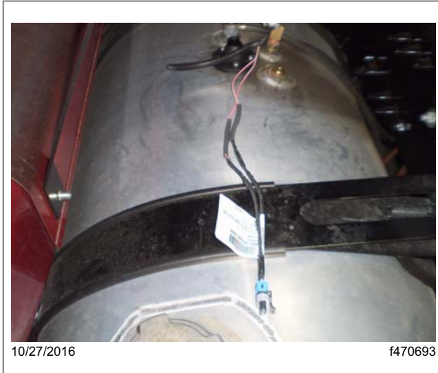
Fig. 6, New Pigtail Installation
