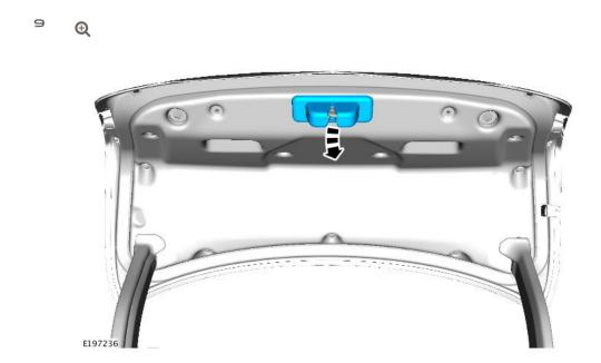
Pull the luggage compartment lid down by pulling on the luggage compartment lid latch cover to confirm the integrity of the installation.
