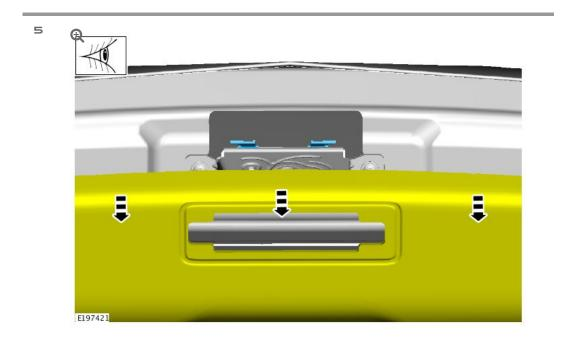
Pull the luggage compartment lid carpet trim down as shown and visually check the latch assembly clipping features are intact and not damaged.
