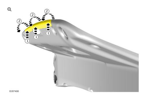
Push in at (1) whilst bending the top edge (2) towards you to flatten any high points on the return edge.
