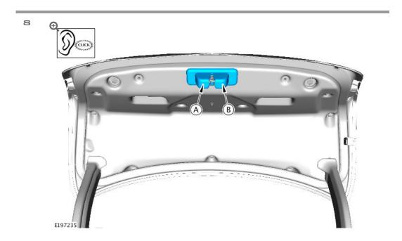
Install the new luggage compartment lid latch cover by pushing with the palm of your hand on the center of the latch cover until a click noise is heard.
