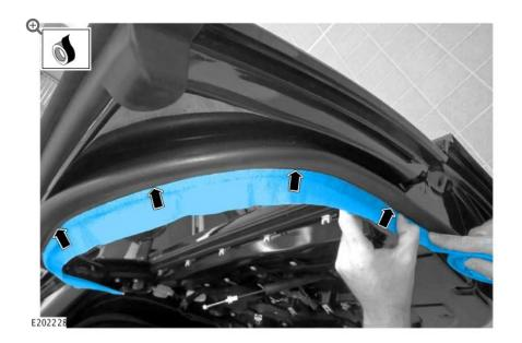
Using a suitable tape, mark the position of the inside edge of the door primary seal following its profile around the whole door.
