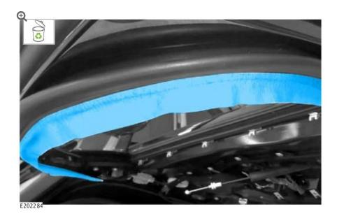
Remove the tape around the door seal.
