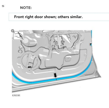
On the lower edge of the door, mark the center position where the two ends of the door primary seal join on the tape already applied.
