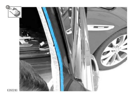
Clean and remove any remaining door seal adhesive from the edge of the door.
