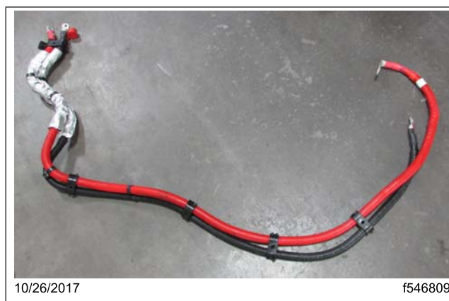
Fig. 4, Positive and Negative Battery Cables Removed
