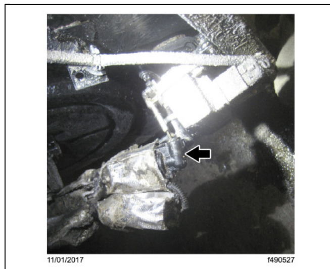
Fig. 1, Broken DEF Line
