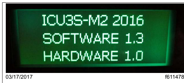
Fig. 1, ICU3S Screen Showing Software Version 1.3 (correct)
