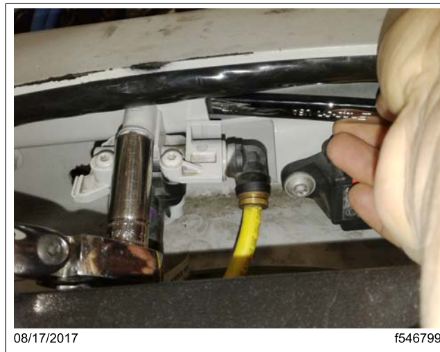
Fig. 3, Wrench Holding the Nut in Place
