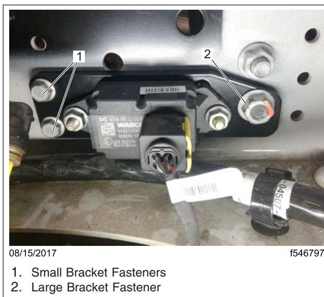
Fig. 7, New ESC Bracket Fasteners
