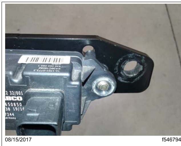
Fig. 6, Installing the ESC on the New Bracket
