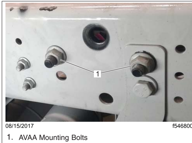
Fig. 10, Crossmember with AVAA Bracket Installed
