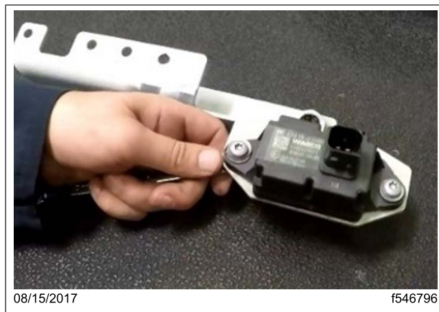
Fig. 5, Removing the ESC Module from the Old Bracket
