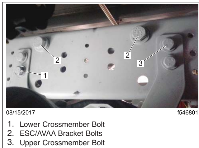
Fig. 4, Crossmember Backside, with the Old Bracket Installed
