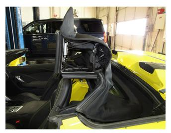
Warning: Due to bleed off of the hydraulic pressure, the folding top will have to be supported or held in mid-position by an assistant. Manual operation of the top cannot be attempted for at least 5 minutes from the last time of activation.
