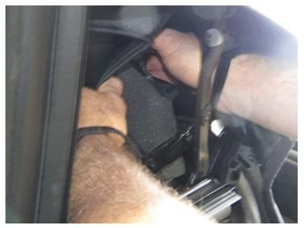
2. Position the top to best reach under the headliner to access the 3 retaining screws on each end of the #3 Bow.
