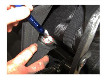
Following the Service Procedure below, remove the original smaller screws and install the new large M6 screws referenced in the Part Table.
