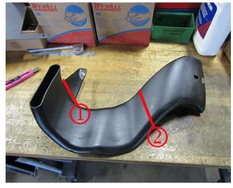
4. Using a hack saw, cut the support arm off (1) and the duct after measuring 50.8 mm (2 in) (2) after the second bend.
