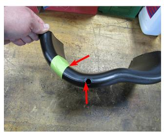
**5.** Measure 50.8 mm (2 in) up from the top of the hole. Mark and cut using a hack saw.
