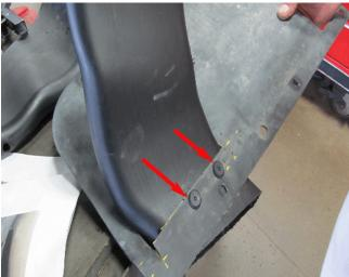
6. Place the cut duct into the slot. Make sure it comes out of the slot 25.4 mm (1 in). Using a 17/64" drill bit, drill 2 holes through the deflector and duct and rivet together.
