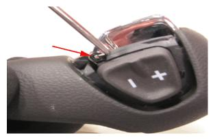
3. Remove the pin located under the chrome knob as shown in the illustration above.
