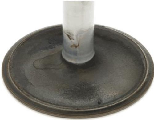
**Engine intake valve using TOP TIER™ Detergent Gasoline having a high detergent treat rate with less than 50 mg deposits.**
