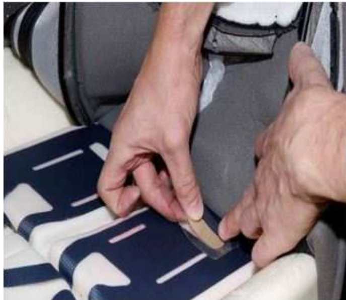
Fig. 4 Installing Patch On Heater Element
