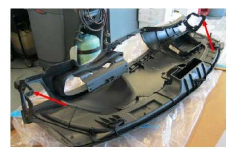
As shown in the photo above, the replacement IP does not include the white insulation material. Although the ductwork does the bulk of holding the insulation in proper position, there are a few places where it is heat-fused as shown in the photo below to the original part. **CAREFULLY** cut around the fuse point with a small utility knife or scissor to release it then pull the insulation away from the original IP taking care to not tear it.
