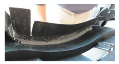
• <u>VERY CAREFULLY</u> using the molded-in groove as a guide, trim the IP as shown to gain access to the square hole for the combination meter top retaining screw clip. After cutting, peel away the trim surface then the foam underneath it to access the square hole for the clip.
