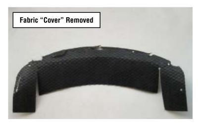
• Once the cover is removed, a **VERY** small amount of black or clear silicone sealer / adhesive works well to "tack" it into position on the new IP. Once in place, a small "fillet" of black or clear silicone can be applied from the back side as shown below to fully secure it in place. (Gray was used for photo.)
