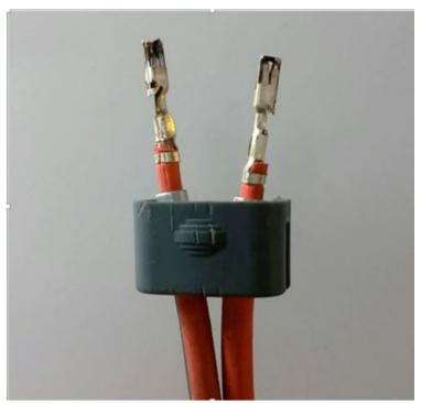
If there is no trouble found with this connection, check other high voltage connectors for intermittent or open circuits.
