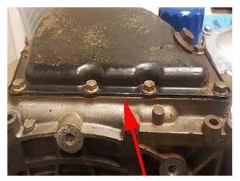
If technician notices an oil leak in between the lower and upper oil pan (red arrow) anywhere around the perimeter, do not attempt to reseal. Contact the engineer listed below prior to completing any repairs.
