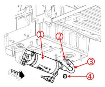
Note: The ground nut can be accessed from under the vehicle and behind the left side rear wheelhouse liner.
