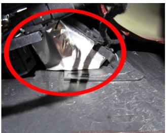
Install a new single piece of aluminum butyl tape on the bottom of the object sensing alert module brackets.
