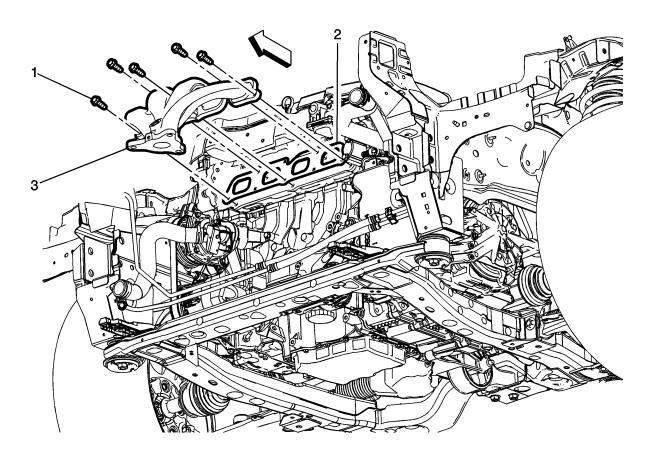
Remove the exhaust manifold (3) and discard the exhaust manifold gasket (2). Refer to Exhaust Manifold Replacement in SI.
