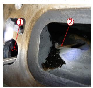
Note: A light and a small pick or screwdriver can be used to validate if the air injection ports are cleared of debris.
