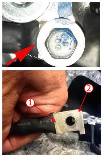
2. Inspect the positive battery cable eyelet at the Power Distribution Fuse Block (UBEC) for either excess heat shrink tubing or glue (1) under the eyelet. Inspect for adhesive that has seeped out onto the eyelet during the heating of the shrink tube (2), or the shrink tube itself extending into the eyelet area. Carefully trim the heat shrink tube if needed, clean adhesive from the eyelet (sand off), reinstall and torque.
