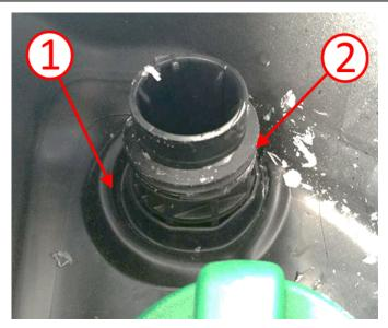
Position the grommet (1) away from the DEF filler cap threads (2).
