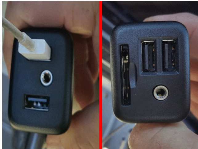
Note: Left Receptacle 2017 Silverado with Radio RPO IOB (Correct), Right Receptacle 2017 Silverado with Radio RPO IOB (Incorrect).
