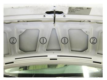
**Note:** The condition is most commonly found at the two center-most inner panels (1), however in some cases the next outboard inner panels (2) may also be affected.
