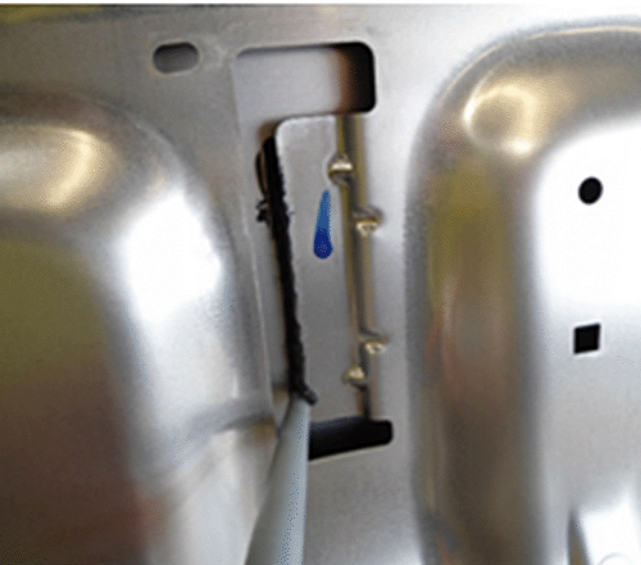
Figure 3 – Apply Henkel Teroson MS 9220 to inner panel tab as shown.
