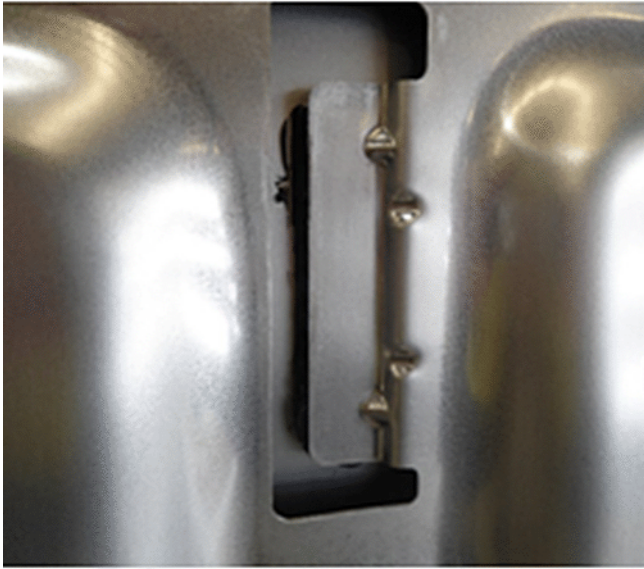
Figure 7 – Appearance of deck-lid inner panel tab at completion of rework
