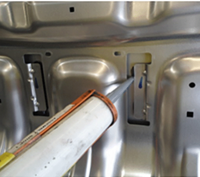
Figure 3 – Apply Henkel Teroson MS 9220 to inner panel tab as shown.
