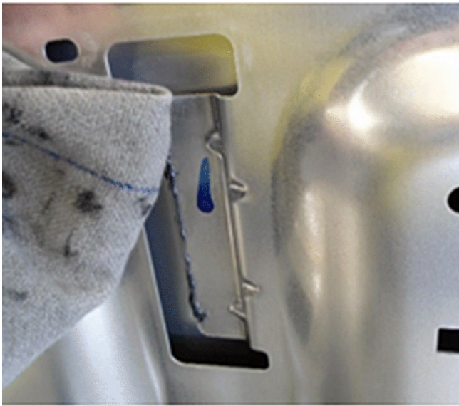
Figure 6 – Wiping excess mastic from the surface
